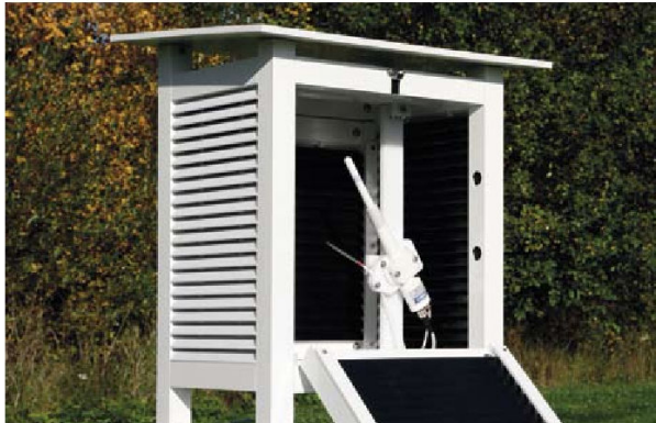
HMP155 with a new, stable HUMICAP®180R sensor and an additional temperature probe.
